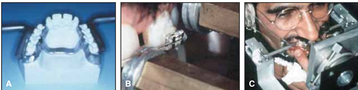
Fig. 1 A. Custom-made partial denture cemented on cast. B. Bonded bracket with archwire and test fixture in place. C. Assembled test fixture allowing measurement of archwire movement relative to bonded bracket and force load. (Reprinted by permission. 61 )
